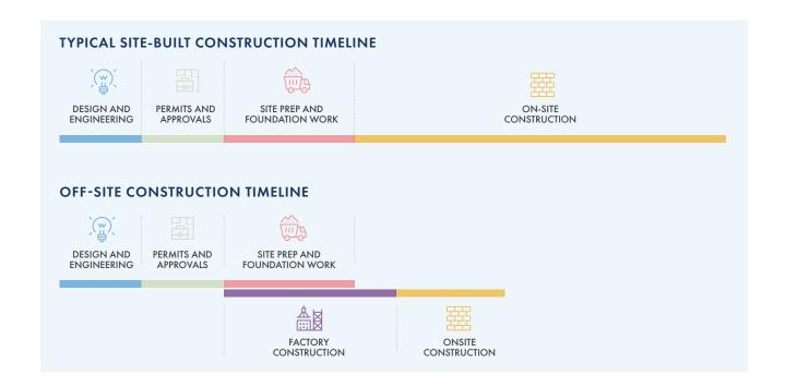
Using off-site construction to develop multifamily housing follows a unique timeline that can offer time-related cost savings.
